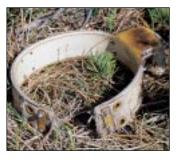
A collar containing the radio transmitter has a cotton spacer that disintegrates after about two years.
